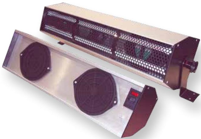
The 935 Ionising Blower provides effective long range ionisation. The Blower comprises an ionisation head and an integrated fan system. A high volume flow of ionised air is generated by blowing air through the ionisation head. Ionisation is provided by powerful 915 Ionising Bars and powered by the 904 Power Supply.
