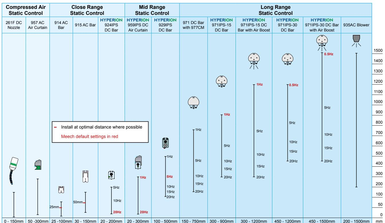
All Meech products have an optimum working distance. These distances vary between our products and the applications they are used in. The chart above highlights the optimum working distance for a range of our static control systems, including the Meech Hyperion™ range, which can be viewed in the Hyperion™ brochure.
