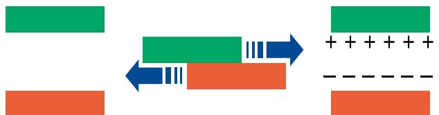
As two materials are rubbed together, the electrons associated with the surface atoms on each material come into very close proximity with each other. Depending on the materials, the surface electrons can be transferred from one surface to another. The transferral and resulting charges created are increased significantly with pressure: the harder the two materials are pressed together, the greater the charge.
