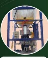
Raising the bottom of the bag into a Steep V shape untying, discharge, bag collapse and removal.
